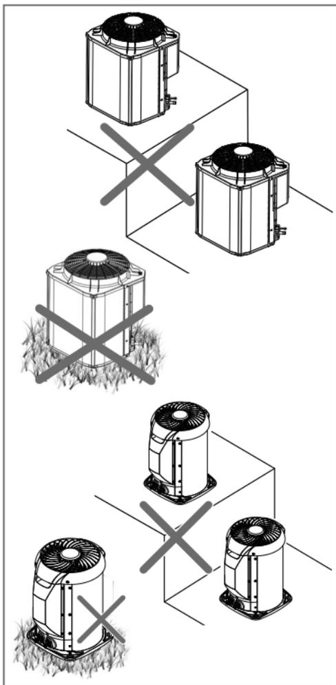
FIG. 3 - EVITAR INSTALAÇÕES
