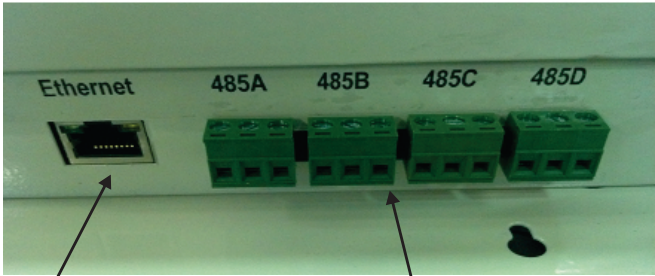
(Ethernet B) Ethernet interface Connect Bacnet/IP network
