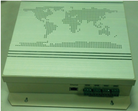
(485A 485B 485C 485D) Four groups 485 interface Each one connects with an indoor Central controller or a outdoor Central controller (F1 F2 E).
