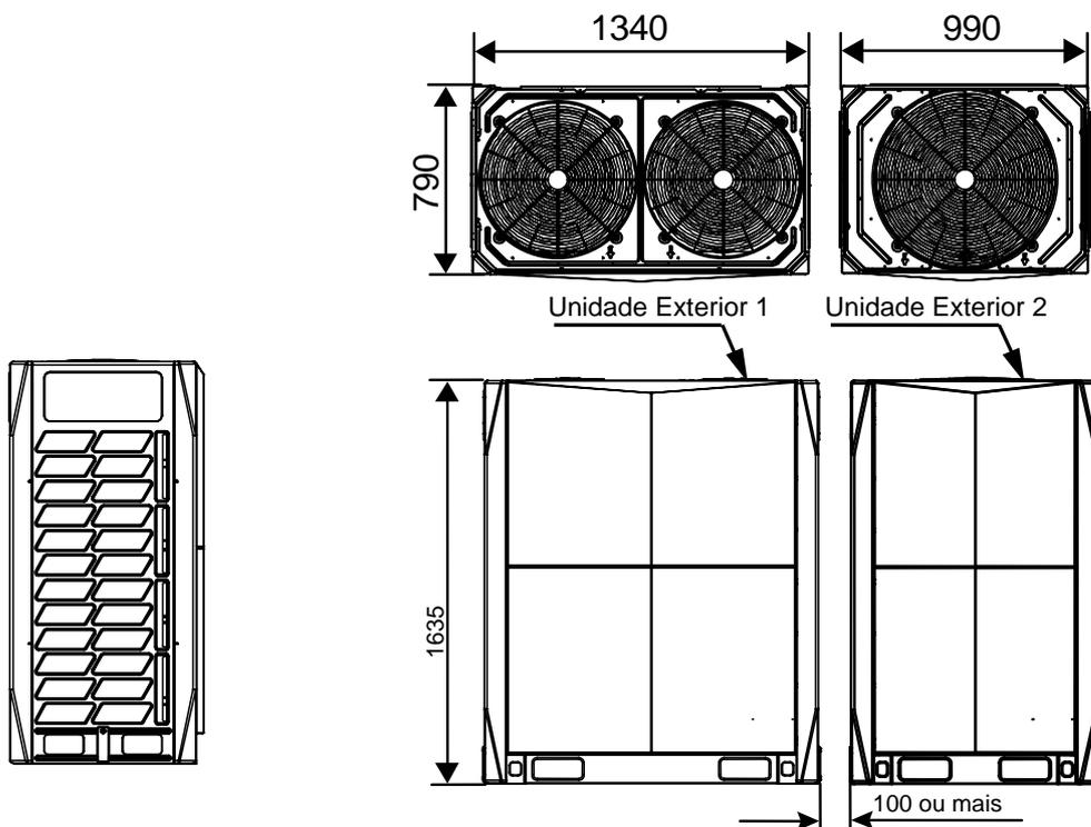
38VF036H119015 / 38VF038H119015 / 38VF040H119015 / 38VF042H119015 / 38VF044H119015
