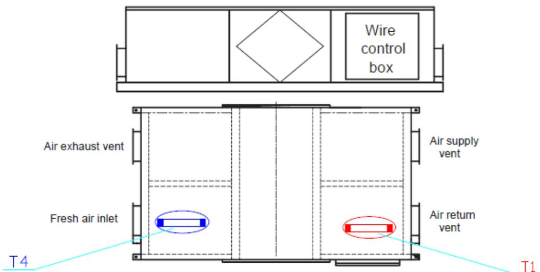
T1 temperature sensor: site at the return air cavity.
