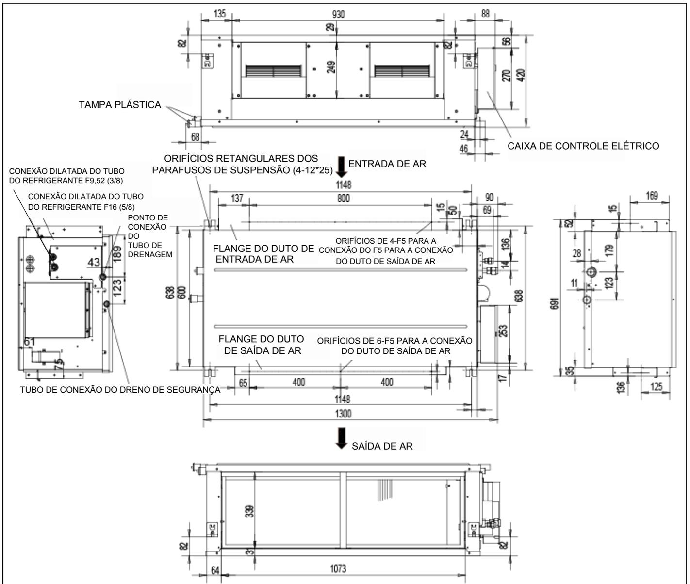
MDV-D200T1/N1-FAA, MDV-D250T1/N1-FAA, MDV-D280T1/N1-FAA
